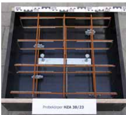
Formwork and reinforcement of test specimen with HZA 38/23
