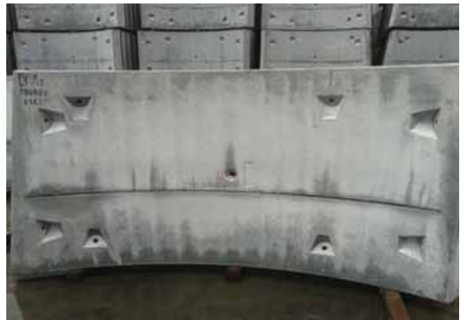
Finished precast segments with cast-in channels
